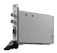
The 52961 NANO-AMP Meter is a single slot PXI module designed to make fast Optical Power measurements and store the results of a sequence of Measurements. The unit has 2 channels for power measurement. Each channel is provided an electrical input connection to allow external photodiodes to be used.
