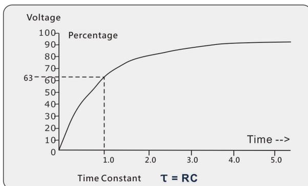
Figure-1 Exponential Response of Voltage across Capacitance
