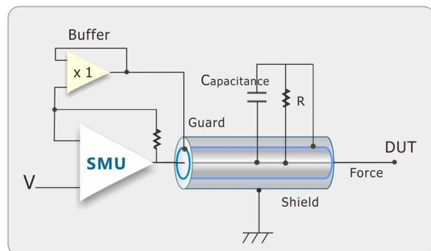
Figure-2 Guard Connection: Cable Capacitance is eliminated with Triaxial Cable
