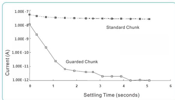
Figure-3 Guarding for IV Measurement Speed
